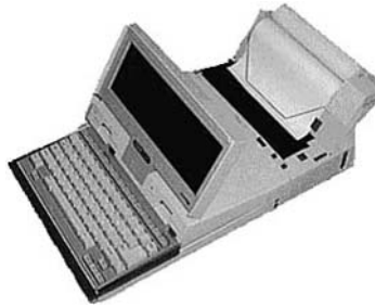
Figure 1.9 The IBM PC Convertible with optional portable printer attached. (Photo from www.can.ibm.com , IBM Canada.)
