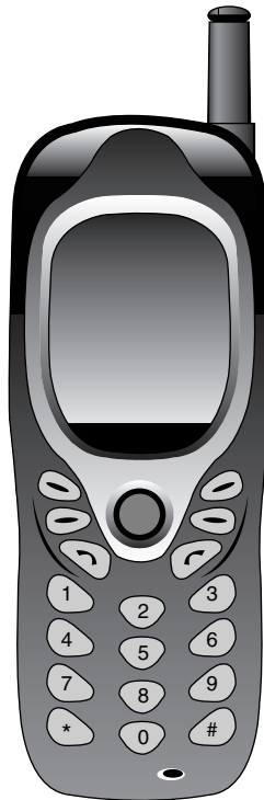
Figure 12.3 The Audiovox CDM8300 Tri-Mode Digital CDMA2000 1X cellular phone, one of many that now include a cellular modem capable of being attached to a laptop.
