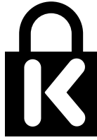
Figure 14.14 The Kensington Lock icon is used to identify security slots on notebooks.
