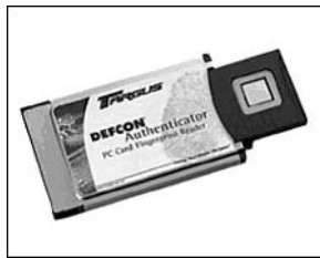
Figure 14.17 The Targus DEFCON Authenticator is a PC Card that has a pop-out fingerprint reader.
