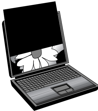
Figure 14.24 The 3M Notebook Privacy Computer Filter limits the visibility of an LCD screen to only the user directly in front of it.
