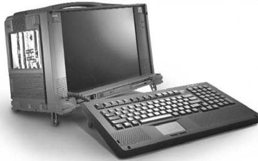
Figure 1.7 The Dolch FlexPAC P4 rugged computer is an example of a powerful lunchbox computer that is still available. (Photo from www.dolch.com .)
