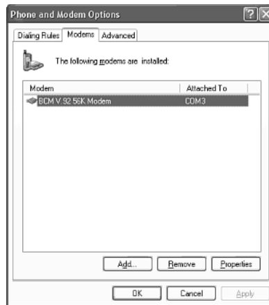
Figure 12.10 A dialog box showing where to find the COM port for a modem under Windows XP.
