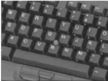
Figure 2.6 The IBM TrackPoint, the original pointing stick. (Photo courtesy of IBM, www.ibm.com .)
