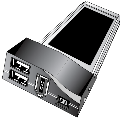
Figure 11.14 The OrangeCombo USB 2/FireWire card includes two USB 2.0 (Hi-Speed USB) ports (left) and a single IEEE 1394a (FireWire) port (center).
