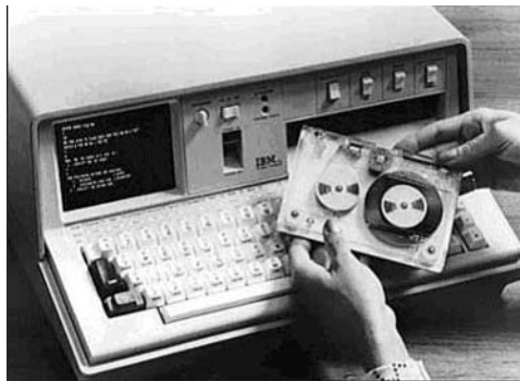
Figure 1.1 The IBM 5100, from 1975. This 50-pound device was the first portable computer, and very nearly the first personal computer. (Photo from www.ibm.com .)
