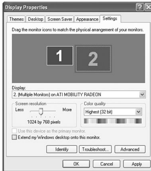
Figure 11.12 The Settings dialog box for a typical laptop with DualView support before the external monitor (monitor #2) is activated.
