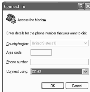
Figure 12.12 The HyperTerminal dialog box showing how to access a particular COM port.
